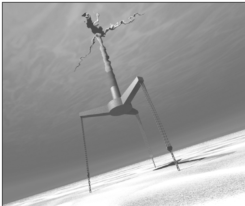
Concept rendering of a tension-leg platform supporting a 5-MW offshore wind turbine in 55 m water depth (fish-eye view) – The Glosten Associates
