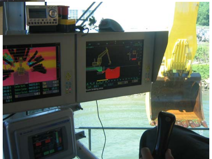
View from operator's cab showing the IHC Systems excavator position monitor.
