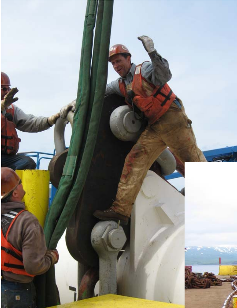
Rigging an intermediate clump weight.
