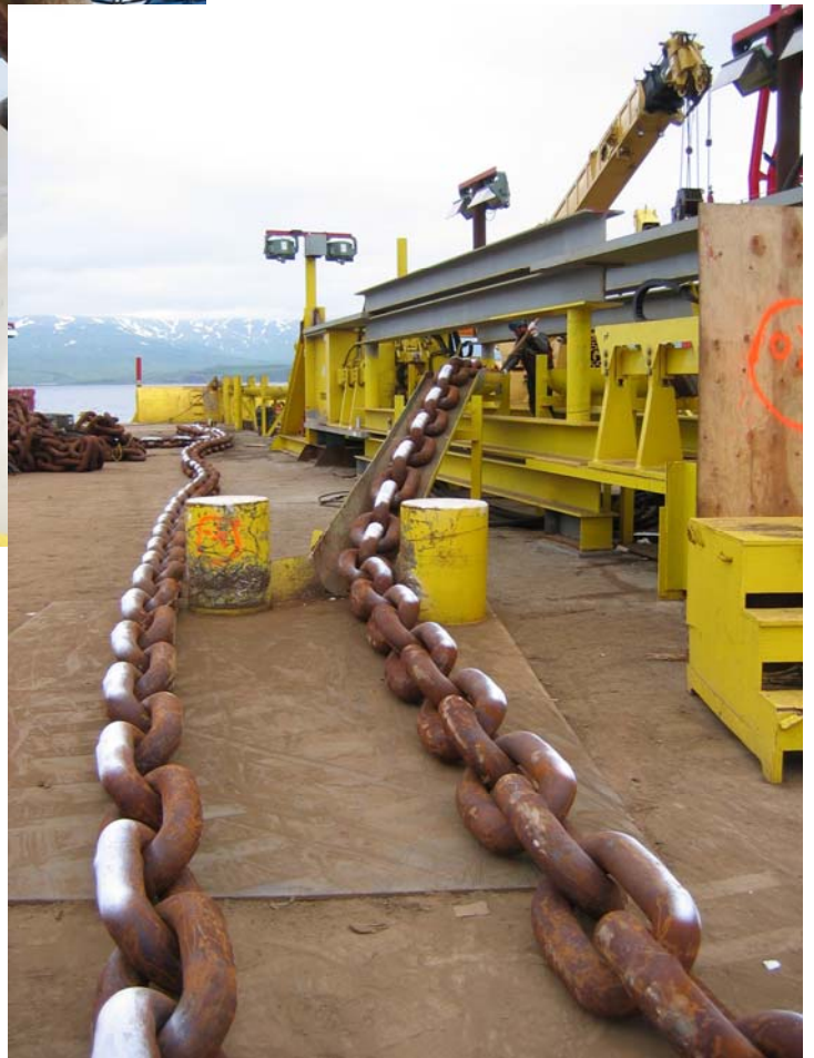
Shown is a test fixture for proof loading opposing anchor pairs to 725 tonnes.
