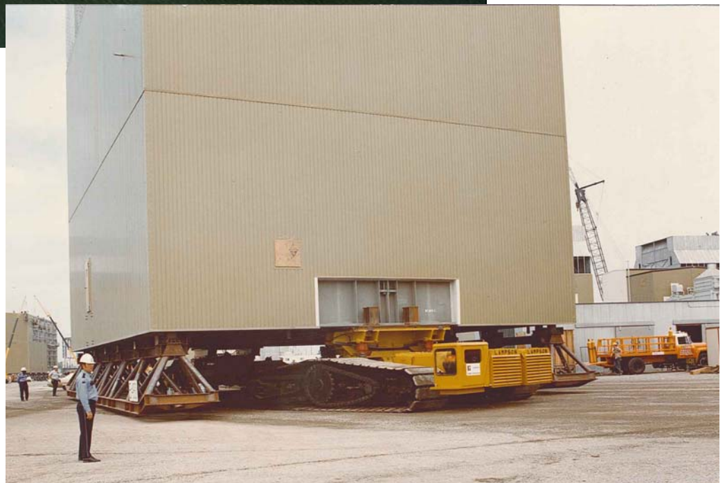
A North Slope process module moving to the Tacoma barge slip on crawler transporters.
