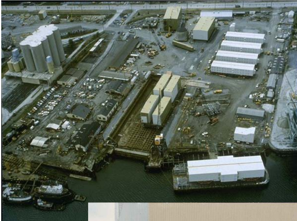
Modules loading aboard barges in a graving dock in Seattle.
