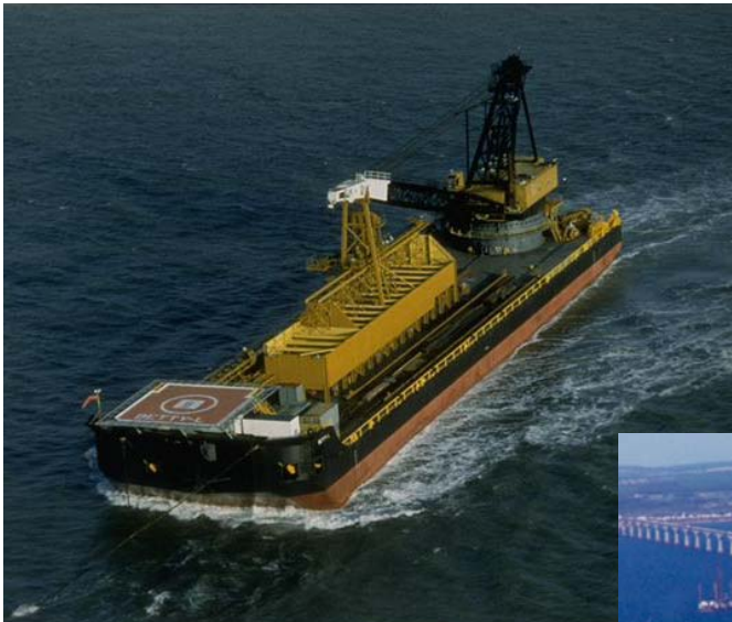
Pictured left is the 6,800 ton, 100 ft x 400 ft Betty L. on her delivery voyage.
